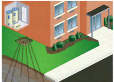
EarthLinked® Water Heating system with diagonal earth loop configuration.
